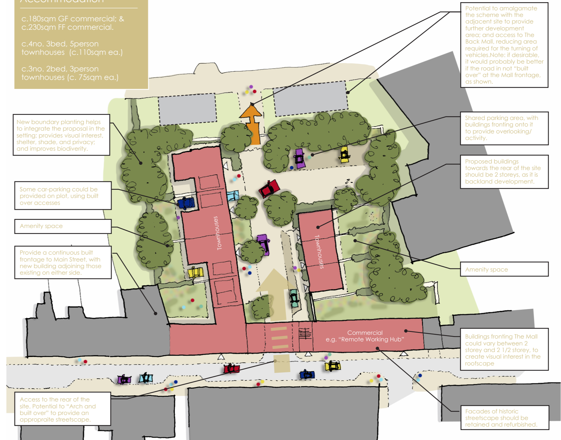
The "Ballyshannon Bakery" site - A conceptual General Arrangement showing one potential option (Mixed-use - Commercial and residential). Alternative uses/layouts may also be appropriate (scale 1:500)
